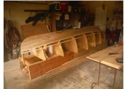
The process continues, first hanging a strake on one side, then the other on the opposite side, then the next set of strakes. After all the strakes are hung, the outer stem and keel are installed. Then the hull is sealed with two coats of thin epoxy, primed and painted. Then it's turnover day!
